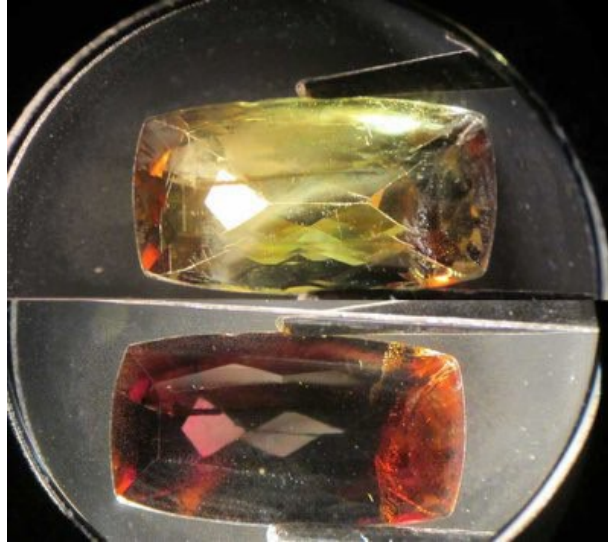
Single andalusite seen through both sides of a London dichroscope.
