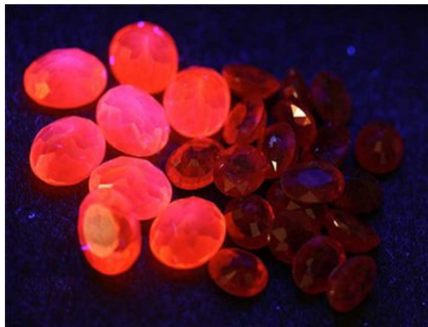
Lab created ruby's reaction brightly to ultraviolet light, while natural rubies on the right stay basically inert.
